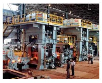
yield strength. The process involves rapid quenching of the hot bars through a series of water jets after they roll out of the last mill stand. The bars are cooled, allowing the core and surface temperatures to equalize. The bar core cools down slowly to turn into a ferrlite-pearlite aggregate. **JAFCO** has been authorized by CRM, Belgium to manufacture Tempcore TMT under licence agreement.
